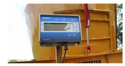
DIGI-STAR 4-POINT SCALE WITH CHOICE OF OPTIONAL DIGI-STAR **MONITORS:** Haybuster CMF's are equipped with the standard Digi-Star 4 Pt. scale and EZ 3500 V monitor. All other Digi-Star monitors and scale heads are available. The Digi-Star system is powered by a standard onboard 12-volt battery. Digi-Star feeding programs are also available. See www.digi-star.com for more information.
