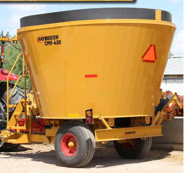
MIXING CAPACITY: The CMF-430 has a 430 cu. Ft. mixing capacity with a tare weight of 10,750 lbs.
