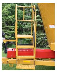
LADDER: Ladder mounted on front of machine allows for viewing of mixed ration while machine is stopped.
