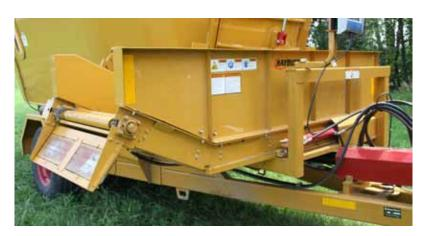
**DOGLEG CONVEYOR:** The dogleg style conveyor hydraulically slides out 16" for easy access to feed bunks.
