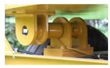
2-SPEED GEAR BOX: The CMF-430 comes equipped with either a Heavy-Duty Constant Velocity 540 rpm PTO or an optional 2-Speed Gear Box. The 2-Speed Gear Box is used for loaded start-ups and heavy rations.
