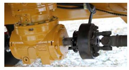
FREE MOTION CLUTCHES ON DRIVELINE: Free motion clutches on driveline protect the heavy duty gearboxes. Gearboxes come with a two-year warranty. The optional two-speed gearbox is used for loaded startups and heavy rations.
