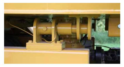
**4-POINT SCALE:** 4-point scale for accurate weighing, with reduced scale bounce during loading and feeding.
