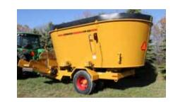
MIXING CAPACITY: The CMF-830 has an 830 cu. ft. mixing capacity with a tare weight of 21,500 lbs.
