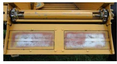
**MAGNETS ON CHUTES:** Magnets on the discharge chutes removes metal, such as bale wire from feed, providing the highest quality feed available. Standard on the dogleg conveyor.
