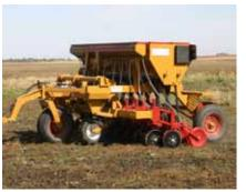
Mechanical Drive System: Wide, aggressive lug-type tractor tire drive wheel, for positive ground contact, to assure accurate planting.
