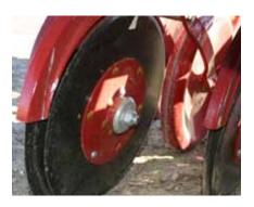
Lead Coulter System: Lead coulter blade is offset 1 ½" in front of dual disc, allowing for cutting of trash and penetrating the soil.
