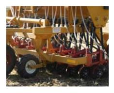
7" Row Spacing: All Haybuster drills plant with 7" spacing and each linkage is offset 9 ½" for planting in heavy residue.
