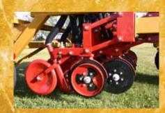
Depth Band: Bolted on to the coulter to limit the maximum seeding depth.
