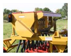
Three Seed Boxes: The Haybuster drills come standard with two seed boxes with individual metering. The third box (front) is the optional legume box. With the legume box installed, Haybuster drills are capable of planting three different seeds at three different rates.
