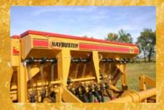
Legume Box: Haybuster drills can be equipped with a third seed box designed for accurately feeding and metering small seeds and legumes. Also available with longer hoses and seed boots for shallow seed placement.
