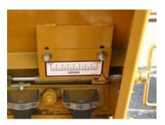
Infinite Seed Rate Adjustment: Easy to set, each box has infinite seed adjustment for accurate seeding rates, no matter what seed you're planting.
