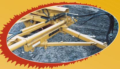
The field and road hitch converts the 3106 Rocke-Eze from road to field and back to road. The field and road hitch centers the 3106 behind the tractor for easier road transport.
