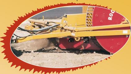
An optional drag plate can be installed when picking rocks on firm soil or in a pasture. The drag plate prevents rocks from being kicked forward onto previously picked ground.
