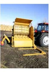
Heavy-duty loader for easy bale loading. Just back into bale, hydraulically rotate shredder frame which loads the bale.
