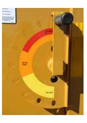
Adjustable slug bars allow you to easily position the bale from the rotor and hammers which also allows you to take any size bite out of the bale
