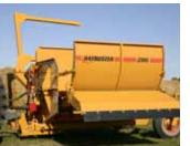
Tractor Semi-Mounted, for easy maneuvering & positioning of straw.
