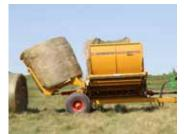
Two-stage bale loader that easily picks up bales without disturbing other bales and gouging the ground.
